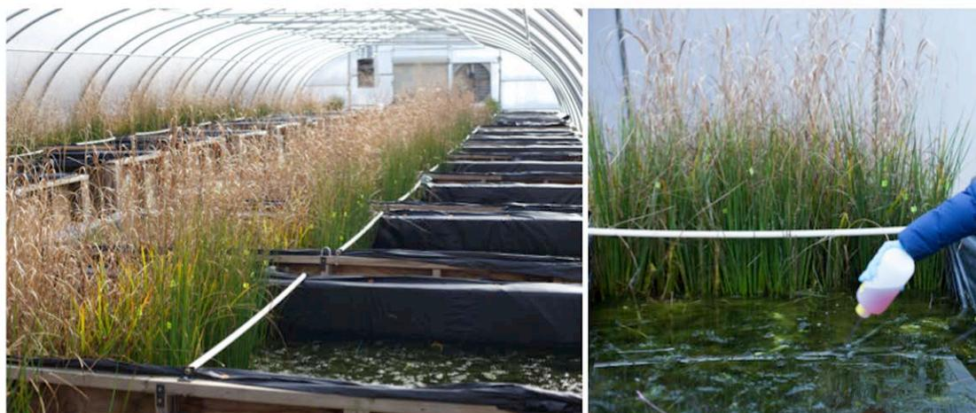
*Left: CEINT mesocosm facility. Right: Weekly dosing of Au NPs.*
