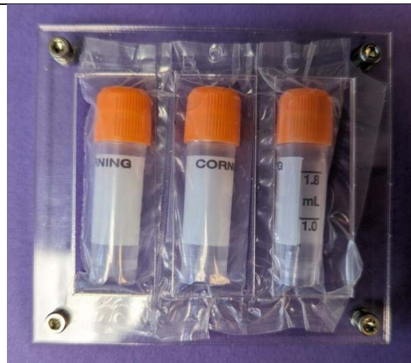
Figure 1. (Top) Sample holder before bagging showing how the sealed liquid sample vials are secured with screws and bolts and pre-cut sample windows. (bottom) Assembled sample holder after heat sealing the sample holder in a bag for a third layer of containment.
