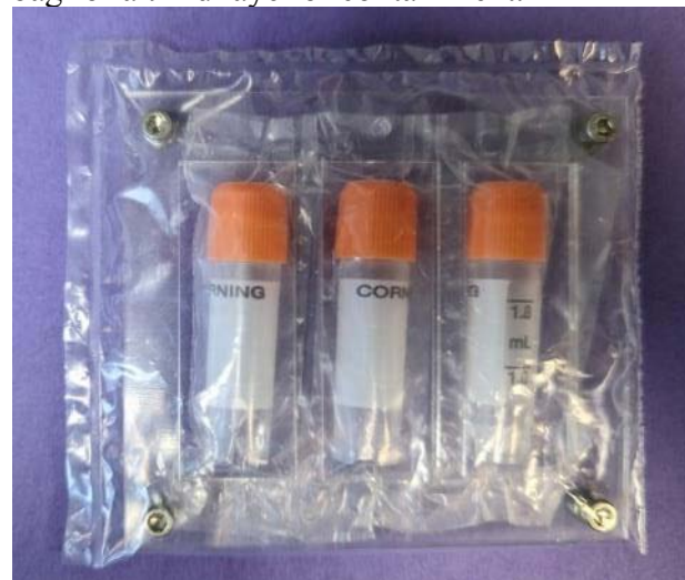
Figure 1. (Top) Sample holder before bagging showing how the sealed liquid sample vials are secured with screws and bolts and pre-cut sample windows. (bottom) Assembled sample holder after heat sealing the sample holder in a bag for a third layer of containment.
