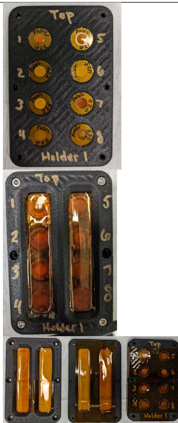
Figure 1. (Top ) Sample holder with Kapton covered stainless steel washers containing sample powder in each of the eight slots. (middle) Assembled sample holder with screws shown at each corner. (Bottom) Image of the front bracket, rear bracket, and sample holder after covering the windows with Kapton tape.
