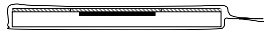
Figure 3. Showing second layer of PP film as an envelope (secondary containment) with a folded and taped tab for closure.
