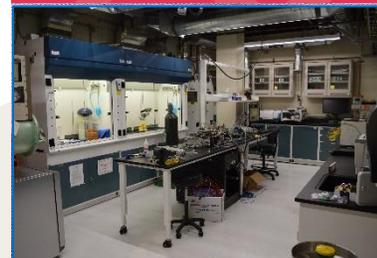
Co-ACCESS operates a 400 ft<sup>2</sup> wet chemistry laboratory specifically designed for catalysis studies. Typical activities in the lab include catalyst synthesis, off-line catalyst treatments, off-line testing of *in-situ/operando* cells for use at the beamlines, and prototyping of catalysis cells. The lab is equipped with
