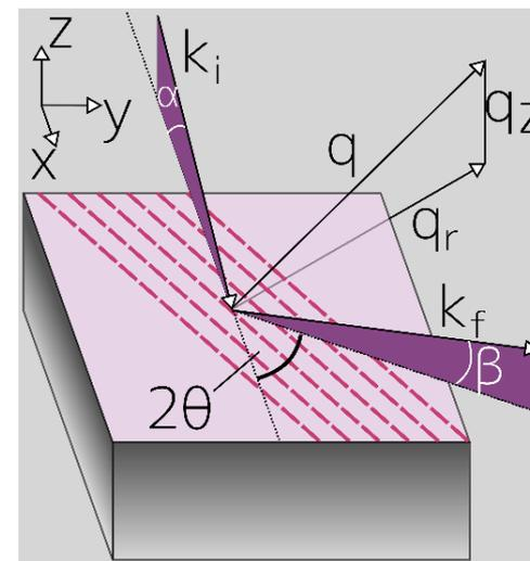
1. X-rays impinge sample under  $\alpha$
