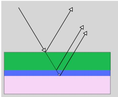
Interference of x-rays reflected from different interfaces → several phase shifts
