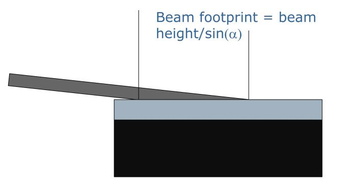
$\alpha$ ~ 0.5, for a 100 micron beam  $\rightarrow$  beam footprint ~10 mm GIXRD requires long ( ~ 20 mm) and flat samples
