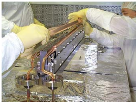
above: BL11-1 1.0m Si flat, side-cooled M0 mirror
