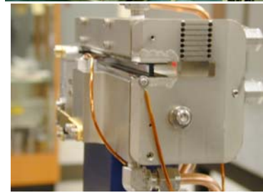
above left - LN mono crystal mount plate above right - two LN monos awaiting installation
