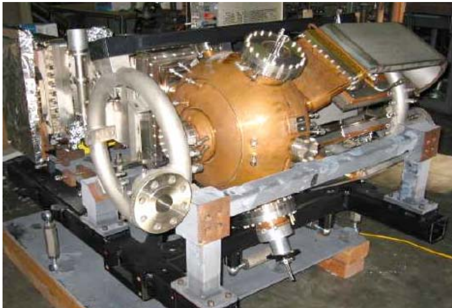
Figure 15 A – SP3 cavity #2 in final assembly
