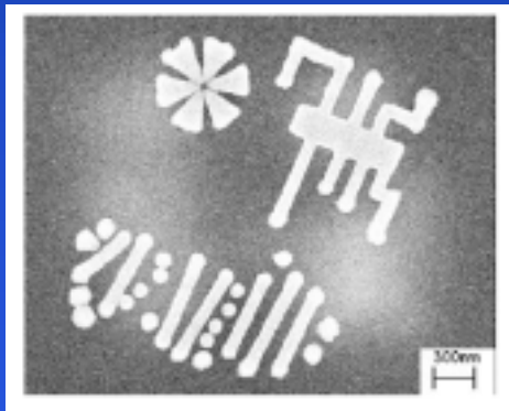
SEM image of Ni pattern on SiN
