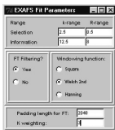
Figure B.3.15: Parameter input box required for performing fits on EXAFS data. This box is created whenever the “EXAFS Fit” radiobutton is active in the “Data Fitting Manager” window.
