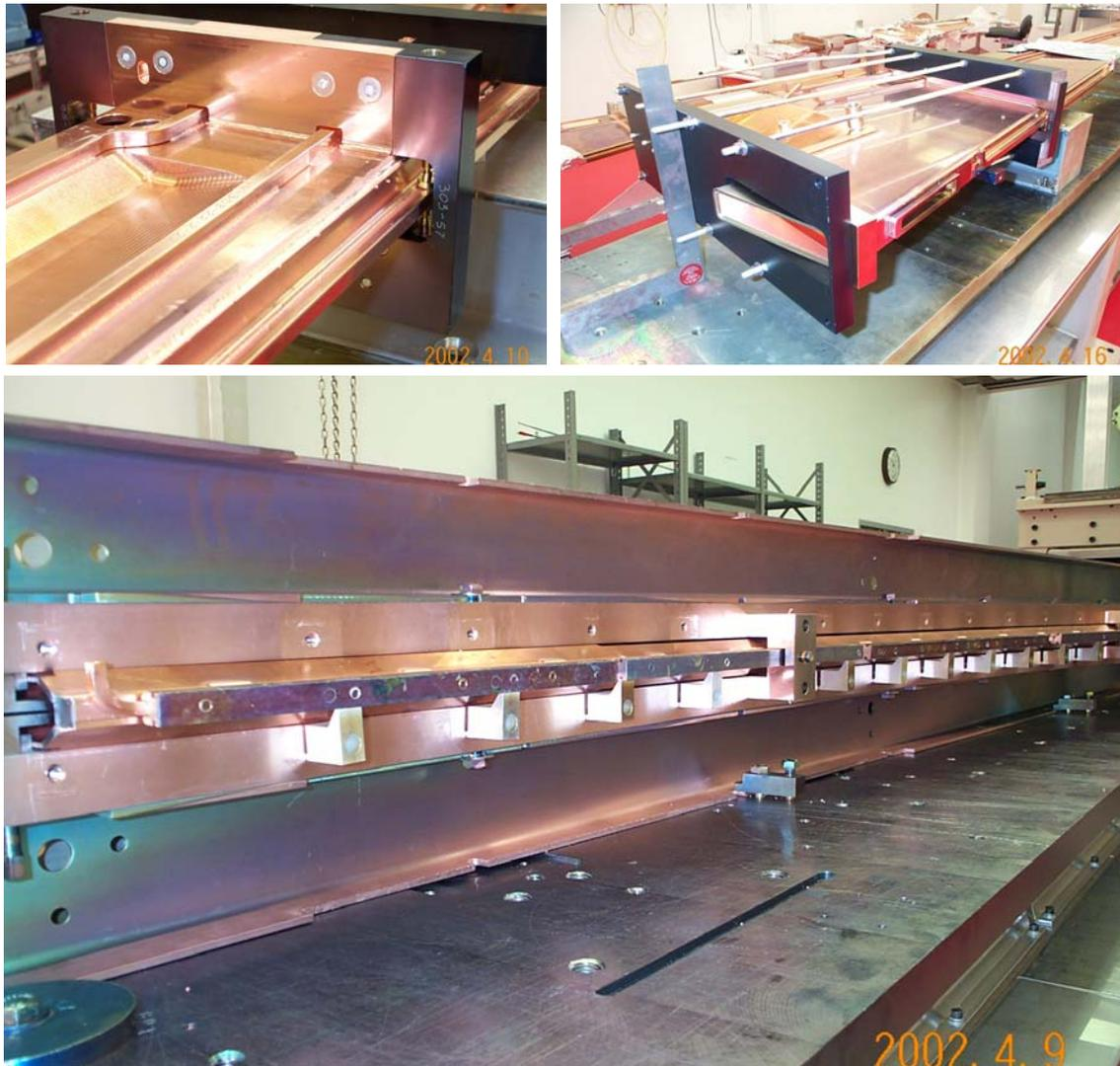
Figure 2.1: BM-1 Chamber Production
