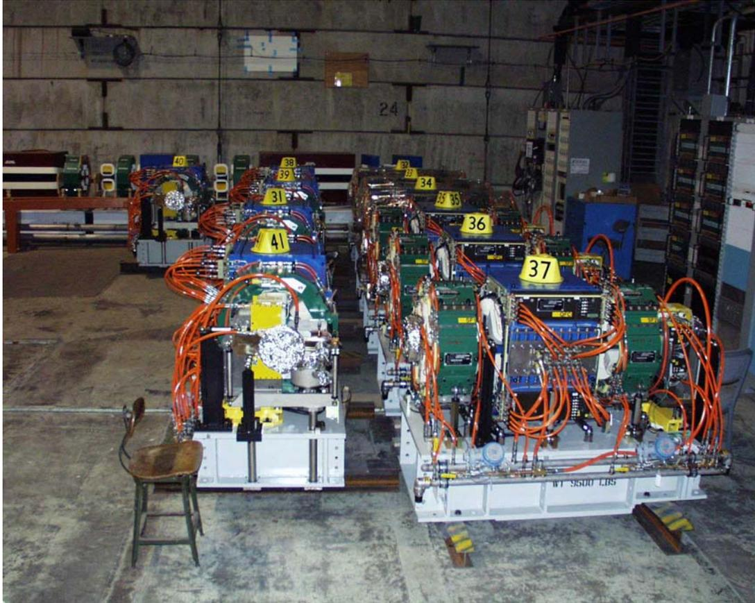
Completed 50Q Rafts in storage waiting for installation into SPEAR
