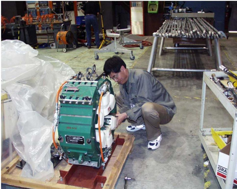
Colleague from IHEP preparing a Sextupole magnet for raft mounting. Note in background are water manifolds for the 145D-Type 2 rafts waiting for assembly.
