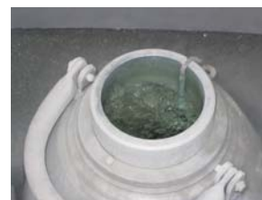
Fig. 2. For shipping dewars containing free liquid nitrogen (hazardous), fill the shipping dewar until liquid nitrogen is observed.
