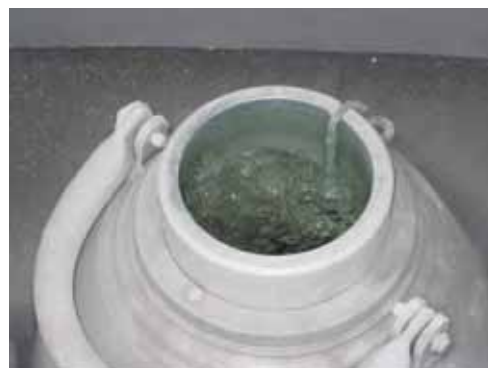
Fig. 2. For shipping dewars containing free liquid nitrogen (hazardous), fill the shipping dewar until liquid nitrogen is observed.
