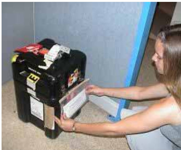
Fig. 3. Attach a plastic envelope containing the proper shipping form to each dewar.
