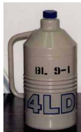
Fig. 1. Designated beamline dewar (4 liters) for filling shipping dewars.
