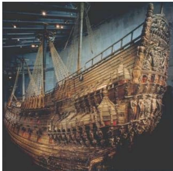
Figure 1. The Vasa on display in the Vasa Museum, Stockholm, Sweden. Dimensions: length 61 m (69 m including bowsprit), maximum width 11.7 m, stern castle 19.3 m high, displacement 1210 tons. (photo by Hans Hammarskiöld at the Vasa Museum). Reproduced by permission, ( http://www.nature.com/ ).
