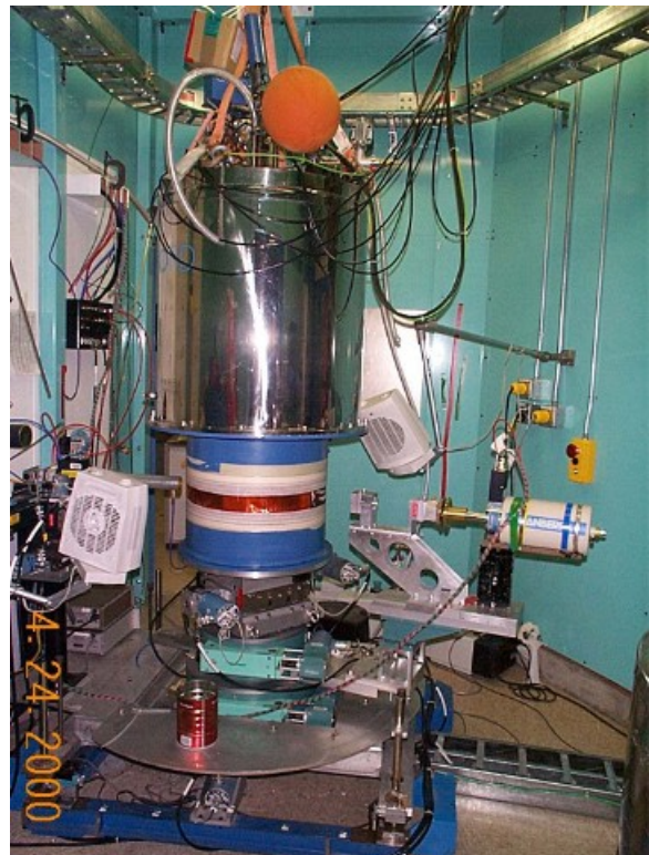
Figure 1. New 13 Tesla magnet facility for x-ray scattering and EXAFS on SSRL beam line BL7-2.
