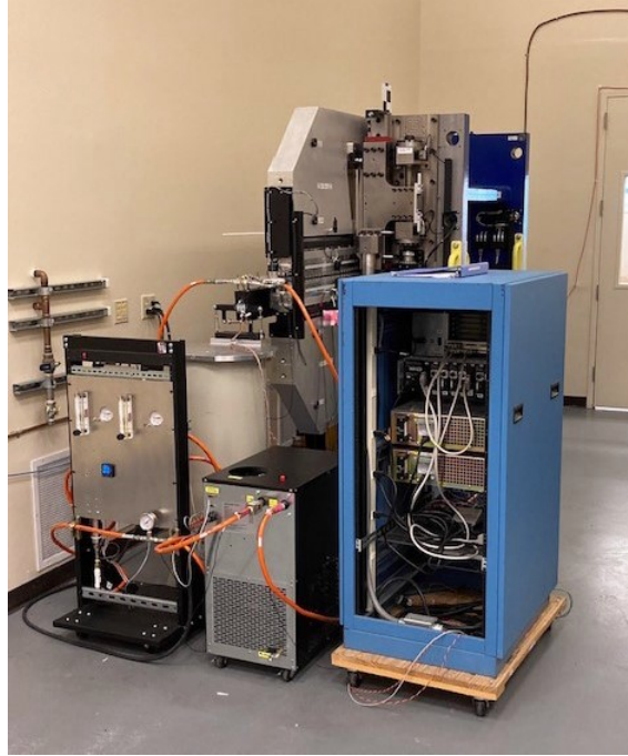
Figure 1: Experimental setup showing the water temperature control system on the left, the water chiller in the middle, a rack with power supplies on the right, and the undulator in the background.
