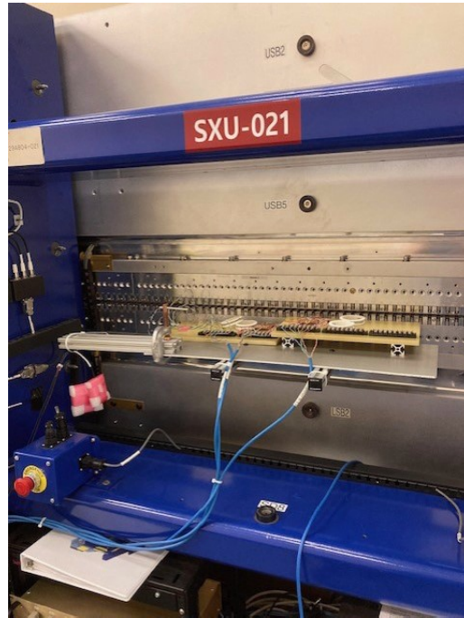
Figure 12: The air temperature reference sensor and monitoring sensor were moved near the thermistors measuring the magnet temperatures.
