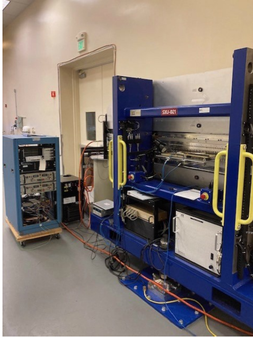
Figure 2: Experimental setup showing the undulator with the thermistor connections near the gap which measure the beam pipe and magnet temperatures.
