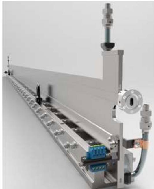
Figure 19: Photo of the HXR undulator beam pipe.
