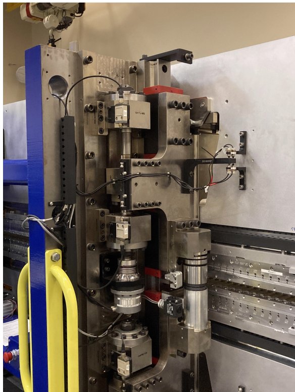
Figure 10: Drivetrain of the downstream side of the upper jaw of HE-SXU-000.
