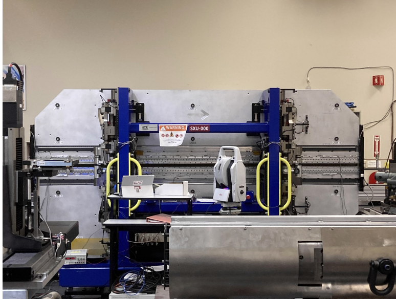
Figure 3: Midplane encoders are mounted inside the blue vertical supports near the top of the undulator.
