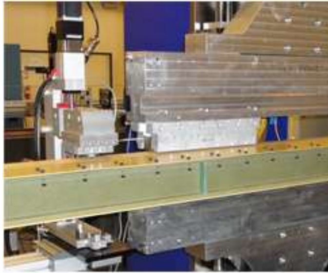
Figure 10: Setup used to measure phase shifter fringe field length.
