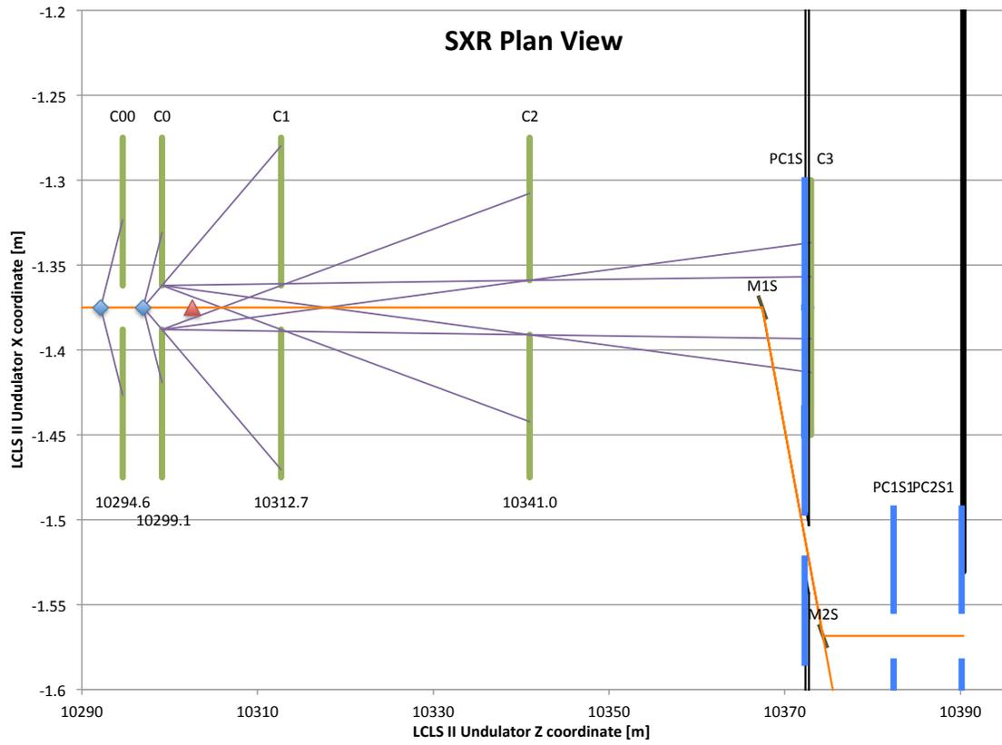
Figure 4: Plan view of the collimators and ray-traces for the SXR beamline.
