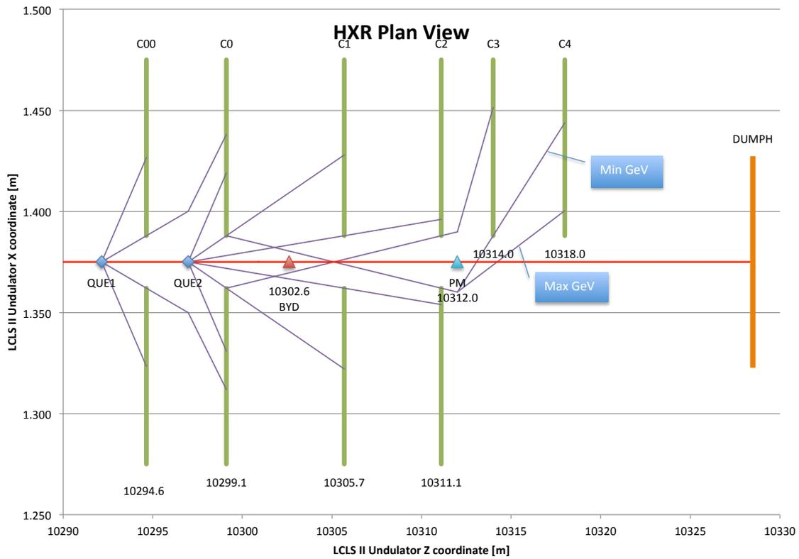
Figure 1: Plan view of collimators (green lines) and ray-traces (purple lines) for the HXR beamline. The horizontally deflecting permanent magnet is represented as a blue triangle. The vertically deflecting electro-magnet is represented by a red triangle.
