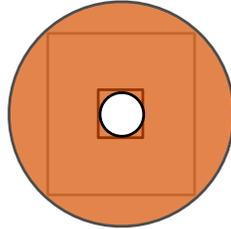
Figure 8: Example of collimator profile that would cover the defined rectangular shape.
