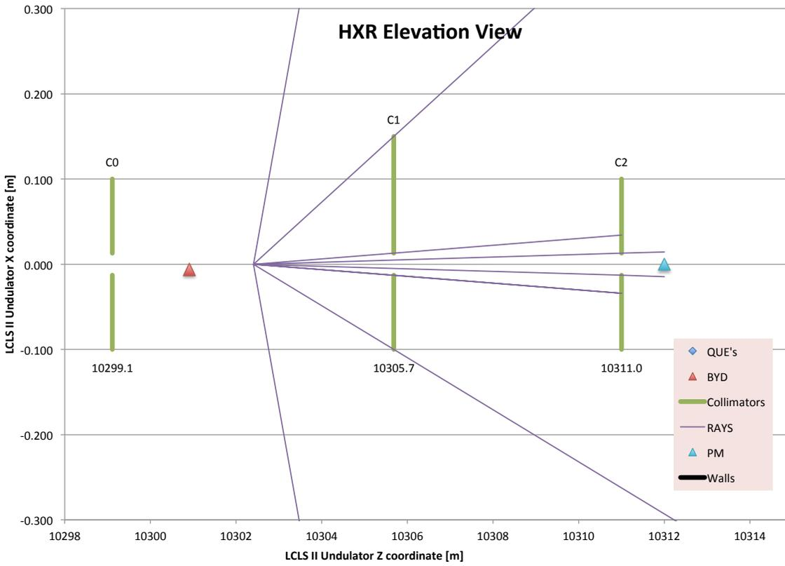
Figure 3: Close-up elevation view of the collimators and ray-traces for the HXR beamline.
