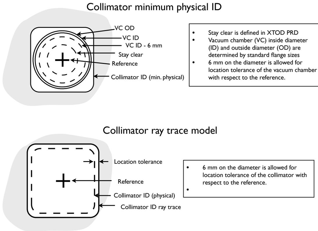
Figure 9: The relationship of the stayclear diameters, collimator physics size requirements and sizes used in the ray-trace study are shown.
