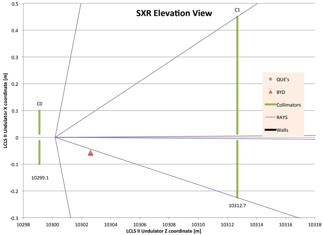
Figure 6: Close-up elevation view of the collimators and ray-traces for the SXR beamline, ceiling, floor, and west wall.
