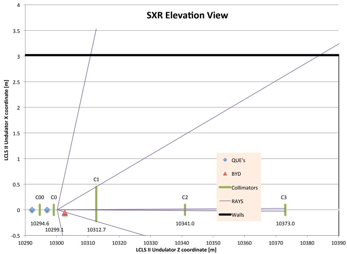
Figure 5: Elevation view of the collimators and ray-traces for the SXR beamline, ceiling, floor, and west wall.
