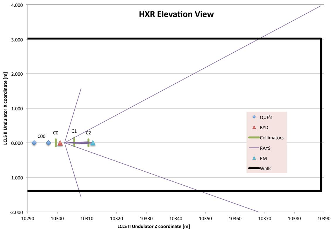
Figure 2: Elevation view of collimators and ray-traces for the HXR beamline.
