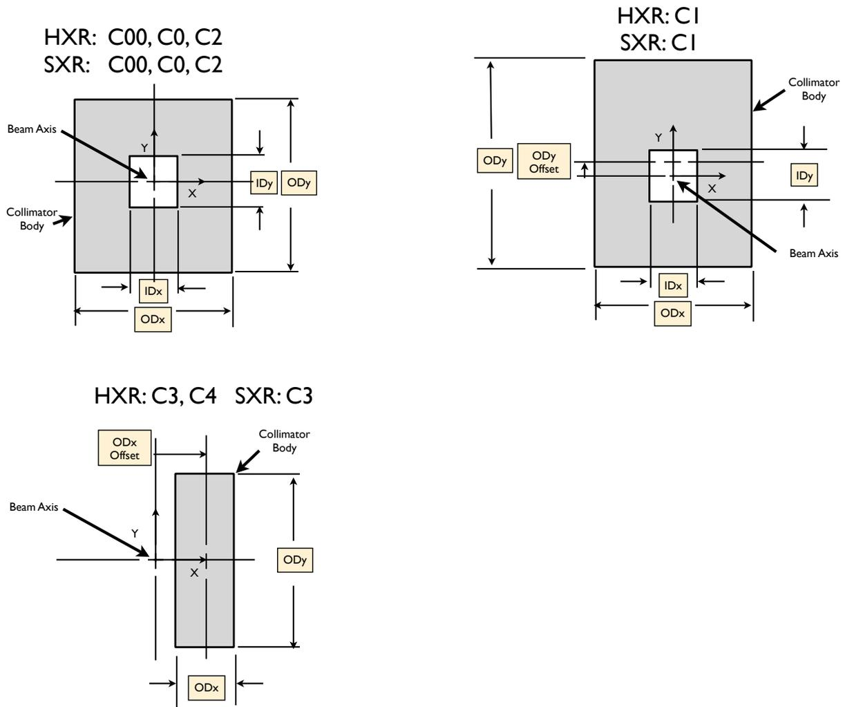
Figure 7: Collimator shape parameter definitions. Coordinates refer to the LCLS-II Undulator coordinate system and the beam is in the Z-direction coming out of the paper.
