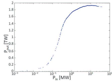
Figure 2: Sensitivity of final FEL power at 160 m as a function of the monochromatized, input seed power as predicted by time-steady GENESIS simulation.
