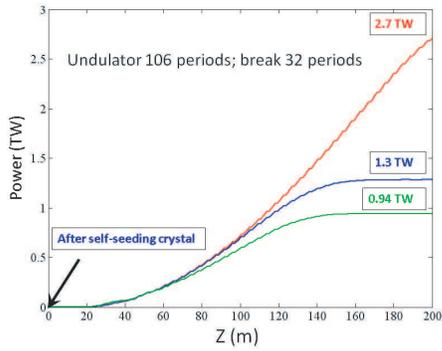
Figure 1: GENESIS predictions for amplification of a 5-MW seed in a tapered, 200-m long undulator for time-steady (red), full time-dependent “fresh” bunch (blue), and start-to-end (green) conditions.
