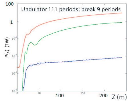
Figure 5: Fundamental (red), 2nd (blue), and 3rd (green) harmonic radiation power vs.  $z$  in an undulator with short break lengths.
