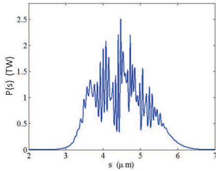
Figure 3: The instantaneous, 8.3-keV power profile at  $z = 160$  m in the second undulator according to time-dependent GENESIS simulation.
