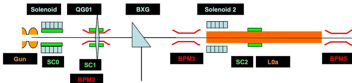
Figure1- Layout of the LCLS injector components from gun to the end of the first accelerating structure.
