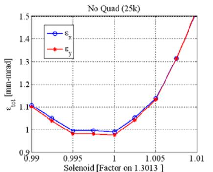
Figure 2 a- No quadrupole component in solenoid
