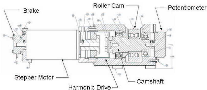
Figure 1: Cross section of roller cam module
