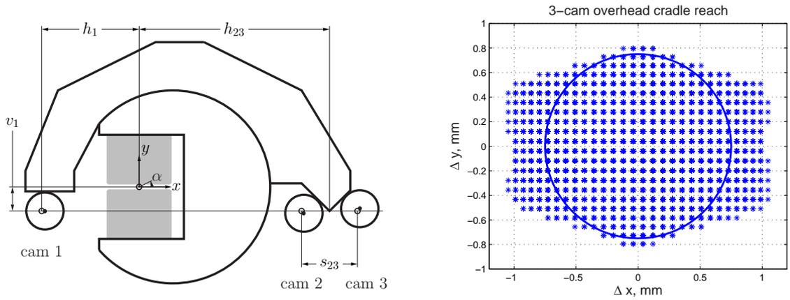
Figure 8: 3-cam overhead cradle decouples roll and  $\Delta x$  motion
