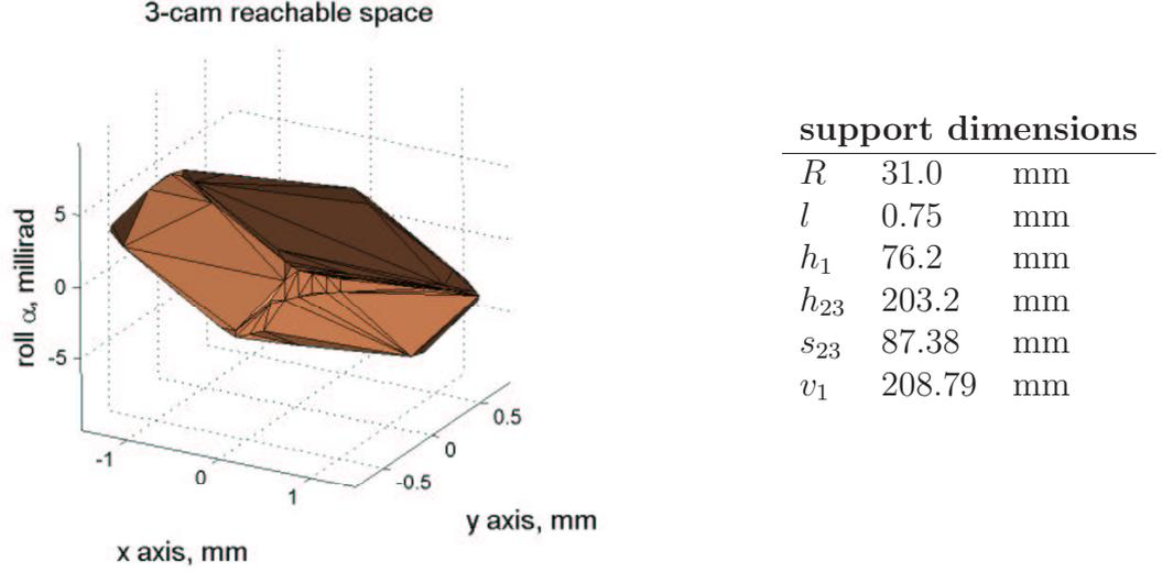
Figure 6: Reachable space for 3-cam support
