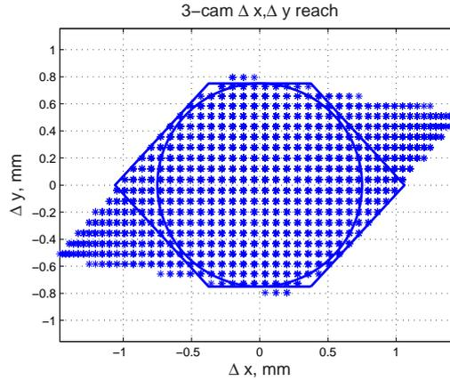
Figure 7:  $\Delta x, \Delta y$  positions reachable by front 3-cam support for all values of roll  $\alpha$ . Cradle support dimensions are same as Figure(6).
