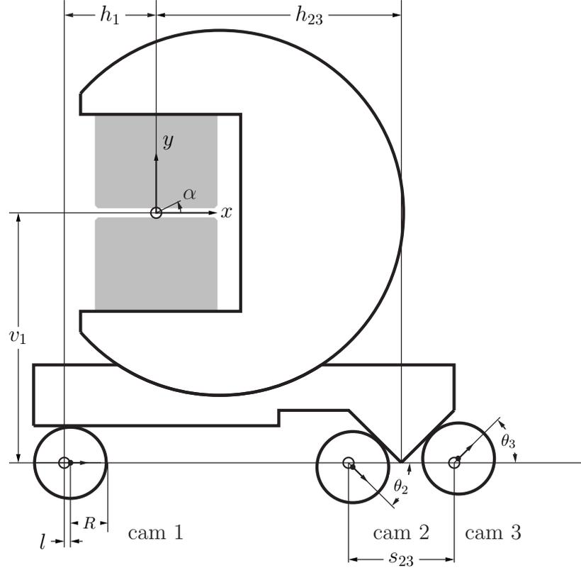
Figure 2: 3-cam undulator cradle in home position with  $x, y, \alpha = 0$ .
