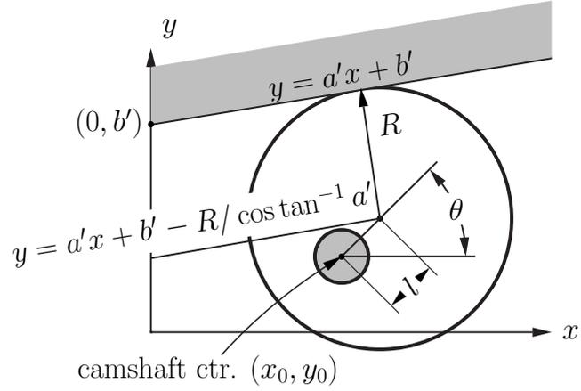
Figure 3: Camshaft angle  $\theta$  for contact between cam radius  $R$  and cradle contact surface specified by line  $y = a'x + b'$ .
