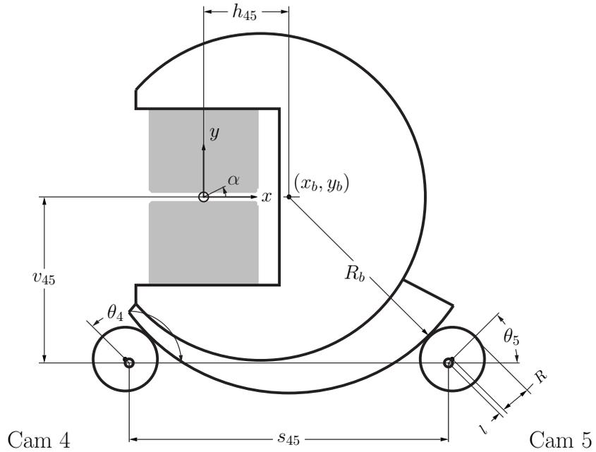
Figure 4: Rear 2-cam cradle support in home position  $x, y, \alpha = 0$ . Cams are placed symmetrically on each side of cradle center  $(x_b, y_b)$ .
