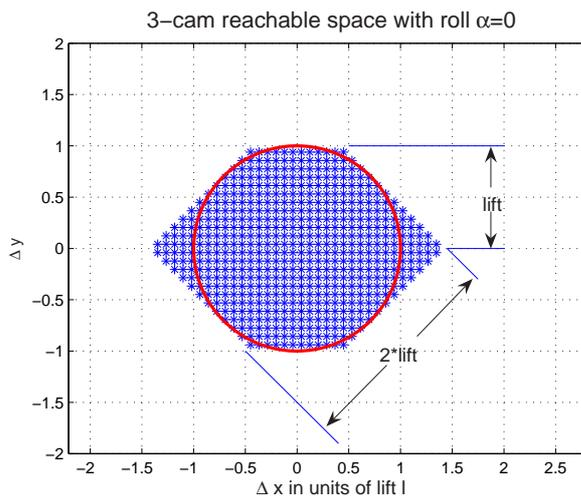
Figure 5:  $\Delta x, \Delta y$  positions reachable by front 3-cam support with roll  $\alpha$  held constant by cam 1. Units are in cam lift  $l$ .
