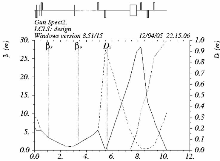
Figure (1)- Optical functions (betatron and dispersion) from TCAV1 to OTRS1 calculated with MAD
