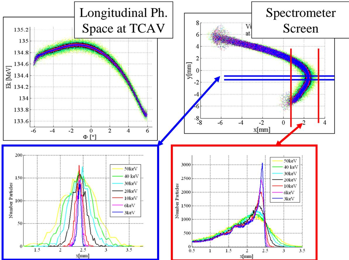
Figure 1 – for nominal beam conditions in the transverse plane but with the uncorrelated rms energy spread increases from 3 to 50 keV - (a) Longitudinal Phase Space at the transverse cavity location –(b) XY image at spectrometer screen- (c) Evolution of vertical slice –(d) Evolution of horizontal slice
