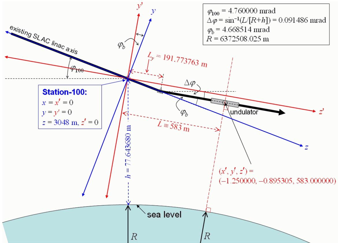
Figure 1: SLAC linac coordinate system  $(x, y, z)$ , and LCLS undulator system  $(x', y', z')$ .
