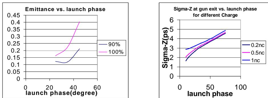
Fig.7: Emittance and bunch length as function of the RF gun phase for 10 ps (FWHM) Gaussian laser pulse. Emittance (cm-mrad) is for 1 nC charge.
