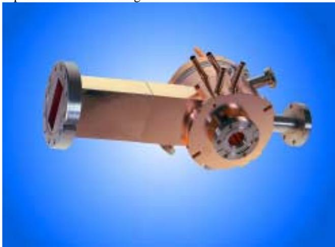
**Fig.1:** BNL photocathode RF gun IV.
