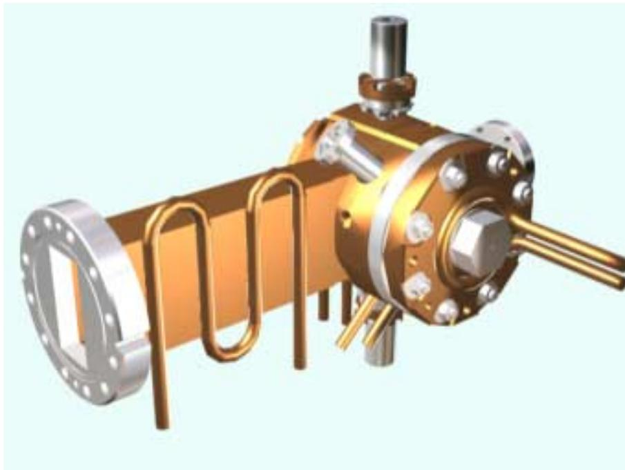
Fig.4: The schematic of 120 Hz RF Gun
