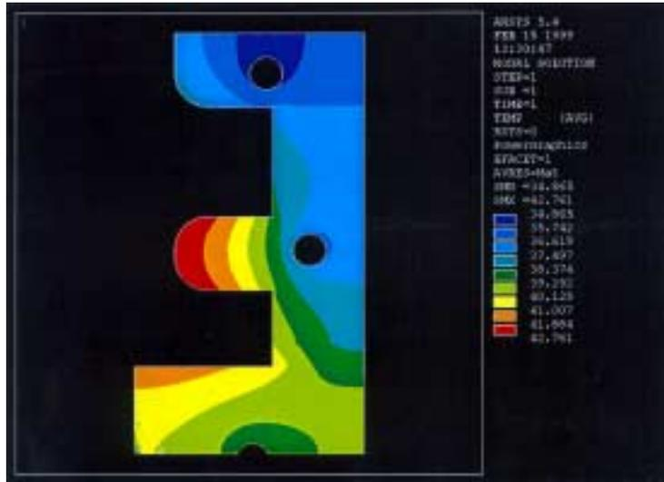
Fig.3: Thermal mapping of BNL Gun IV for 1 KW CW power.
