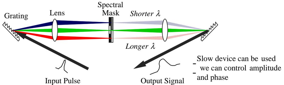
Fig.8: Longitudinal laser pulse shaping using spectral mask.
