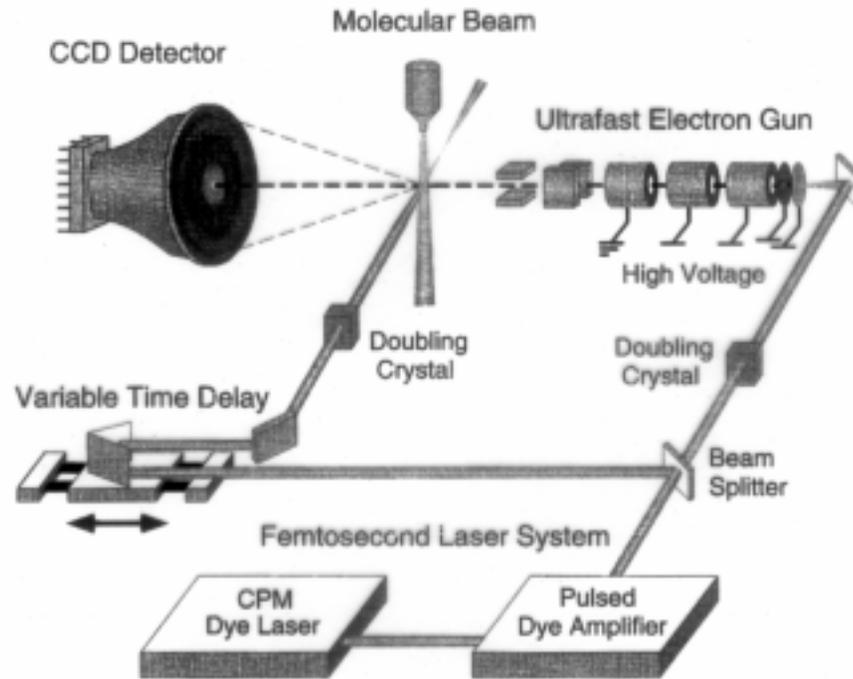
Fig. 1. A schematic of the experimental setup used here for ultrafast electron diffraction (UED).
