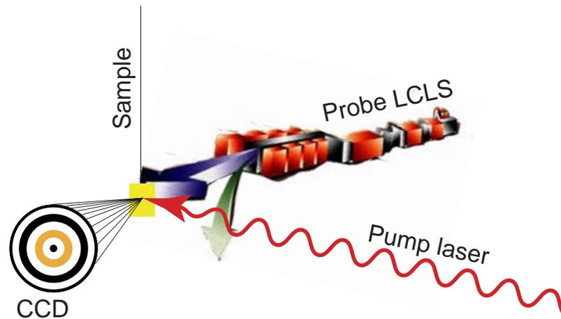
The femtochemistry experiments use an ultrafast laser to initiate the process and the **LCLS** beam as a probe
