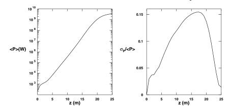
Fig. 4. Evolution of the average emitted power along the wiggler (left) and of the relative power fluctuations along the wiggler (right).
