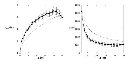
Fig. 1. Half width of the autocorrelation function (left) and power spectrum halfwidth (right) computed from a series of 2D GINGER runs (solid line and dots with error bars) and the predictions of the 1D analysis (dashed line).
