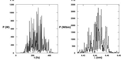
Fig. 2. Temporal structure (left) and spectrum (right) of the output radiation pulse of the TESLA SASE FEL.
