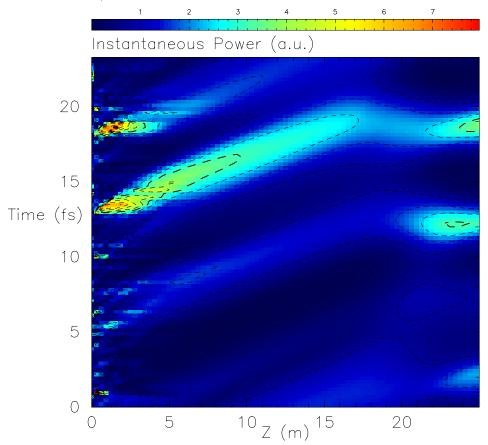
Fig. 3. Plot of the normalized radiation intensity as a function of the wiggler length (horizontal axis) and of the time along a reference frame moving at the ligth velocity, c (vertical axis). For a description of the figure please refer to the text.
