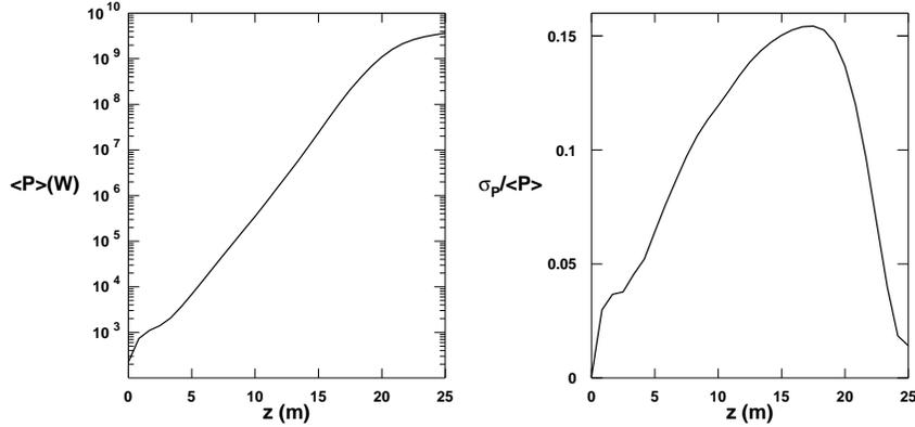
Fig. 4. Evolution of the average emitted power along the wiggler (left) and of the relative power fluctuations along the wiggler (right).
