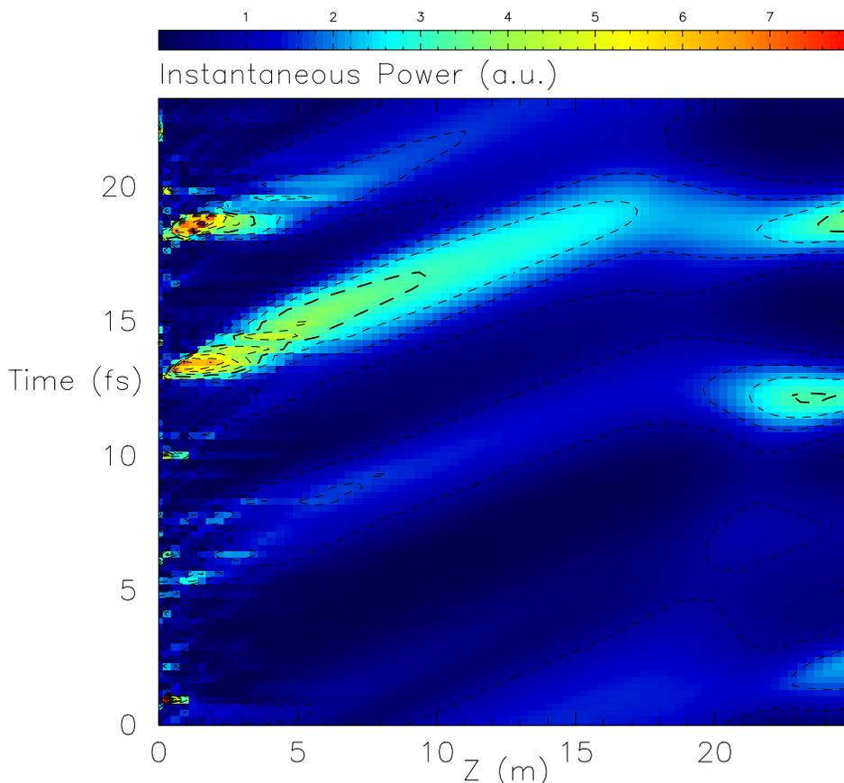
Fig. 3. Plot of the normalized radiation intensity as a function of the wiggler length (horizontal axis) and of the time along a reference frame moving at the light velocity,  $c$  (vertical axis). For a description of the figure please refer to the text.
