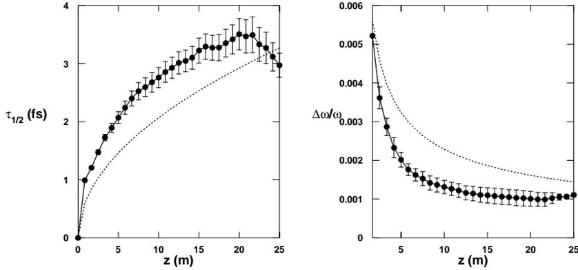
Fig. 1. Half width of the autocorrelation function (left) and power spectrum halfwidth (right) computed from a series of 2D GINGER runs (solid line and dots with error bars) and the predictions of the 1D analysis (dashed line).
