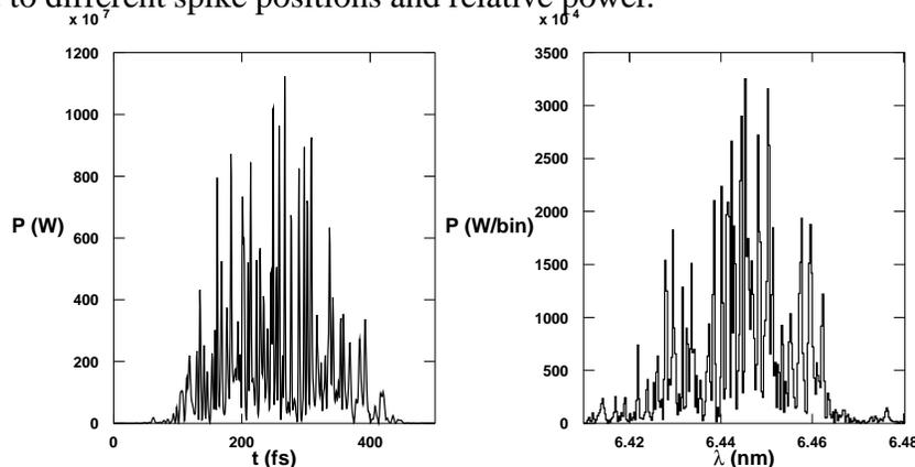
Fig. 2. Temporal structure (left) and spectrum (right) of the output radiation pulse of the TESLA SASE FEL.
