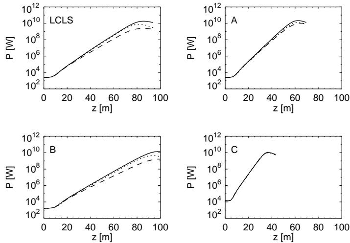
Fig. 2. Radiation power for the different cases including no wake fields, resistive wall wake fields and resistive wall + surface roughness wake fields (solid, dotted and dashed line, respectively).
