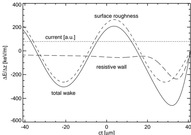
Fig. 4. Wake potentials for the LCLS undulator.
