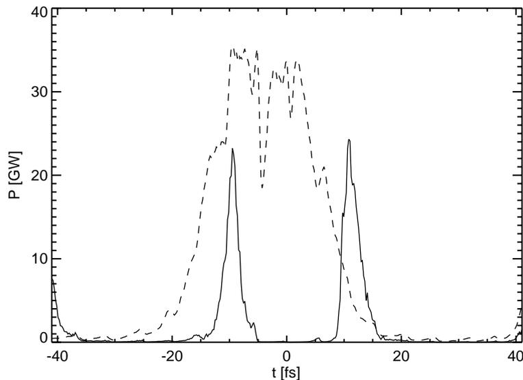
Fig. 5. Average radiation envelope for the LCLS case and case A (solid and dashed line, respectively) close to saturation.
