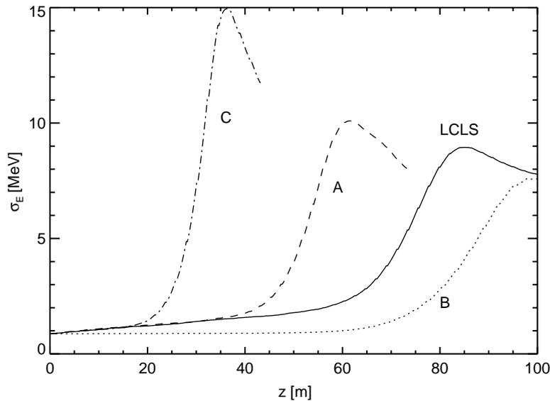
Fig. 3. Energy spread along the undulator including the effect due to the fluctuation of the emitted photons in the spectrum of the spontaneous emission.
