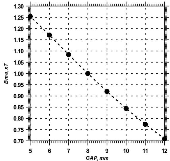
Fig. 1. On-axis field strength versus gap for the Kurchatov design of the helical undulator.
