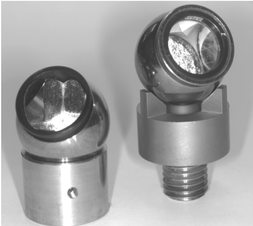
Figure 12.4 Sphere mounted glass and air reflectors
