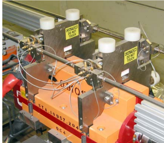
Figure 12.12 Wire Position Monitoring System
