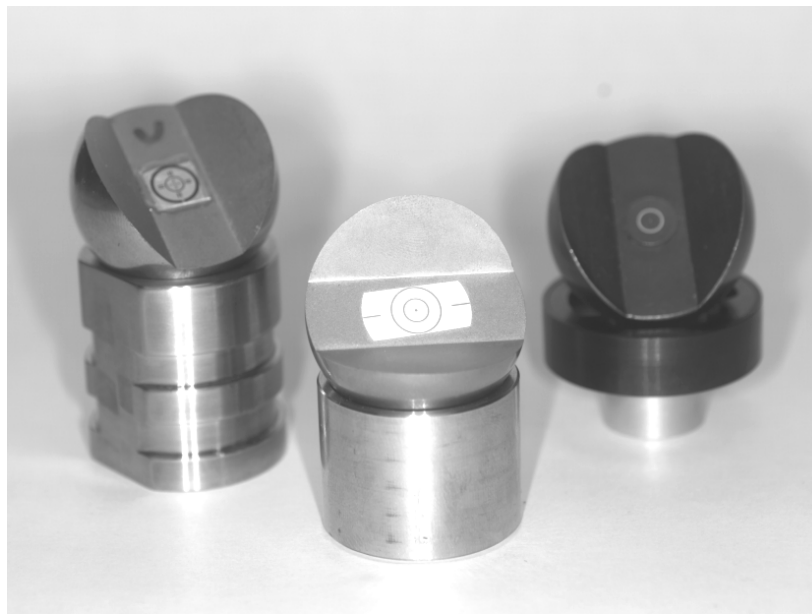
Figure 12.3 Sphere mounted theodolite targets
