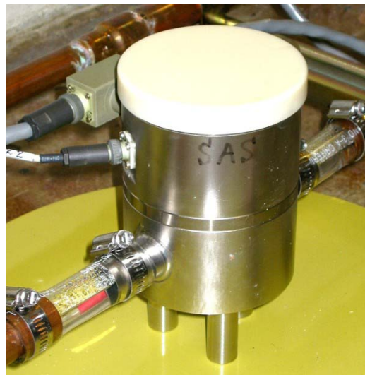
Figure 12.13 “Half-filled” pipe HLS Sensor
