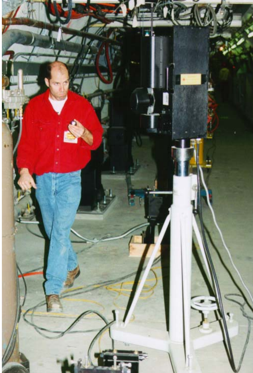
Figure 12.8 Target operator carries the SMX laser tracker reflector.
