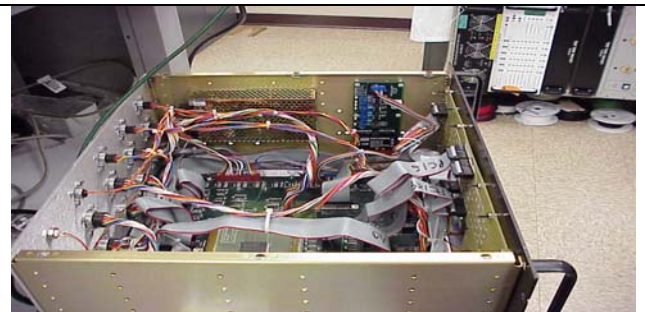
Picture 4.4b New current loop receiver board mounted in the chassis (far side panel)
